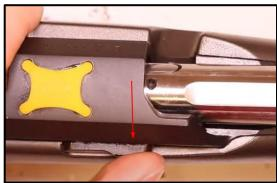
Step 23:Perform a Function Check. Test your Bolt, Safety and Trigger Pull.
