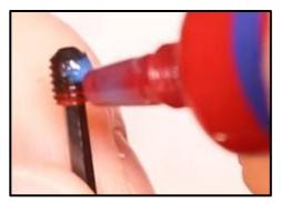
Step 14: Insert the Set Screw back into the Trigger Mechanism.
