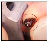
Step 10: Insert your 1/16" Punch where the Set Screw was and Push up on the Coils of the Spring to Compress it out of Place. Then Remove the Spring.
