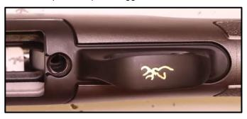
Step 20: Reinsert the Two Takedown Screws. Insert the Longer Takedown Screw in the Hole by the Trigger Guard.
