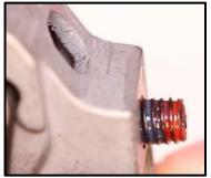
Step 15: Tighten the Set Screw One Full Turn at a Time until there is Roughly Three Threads Showing.
