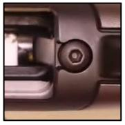
Step 22: Reinsert the Bolt. Hit the Bolt Stop and Let the Bolt Slide in.
