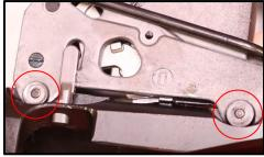
Step 18: Drop your Stock back over the Receiver. Line up the Barrel Lug with the Cutout on the Bedding.
