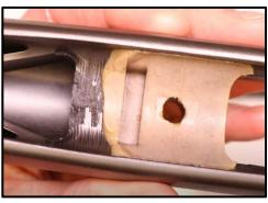
Step 7: Use your 1/16" Punch to Tap out the Trigger Mechanism Pins from Left to Right.
